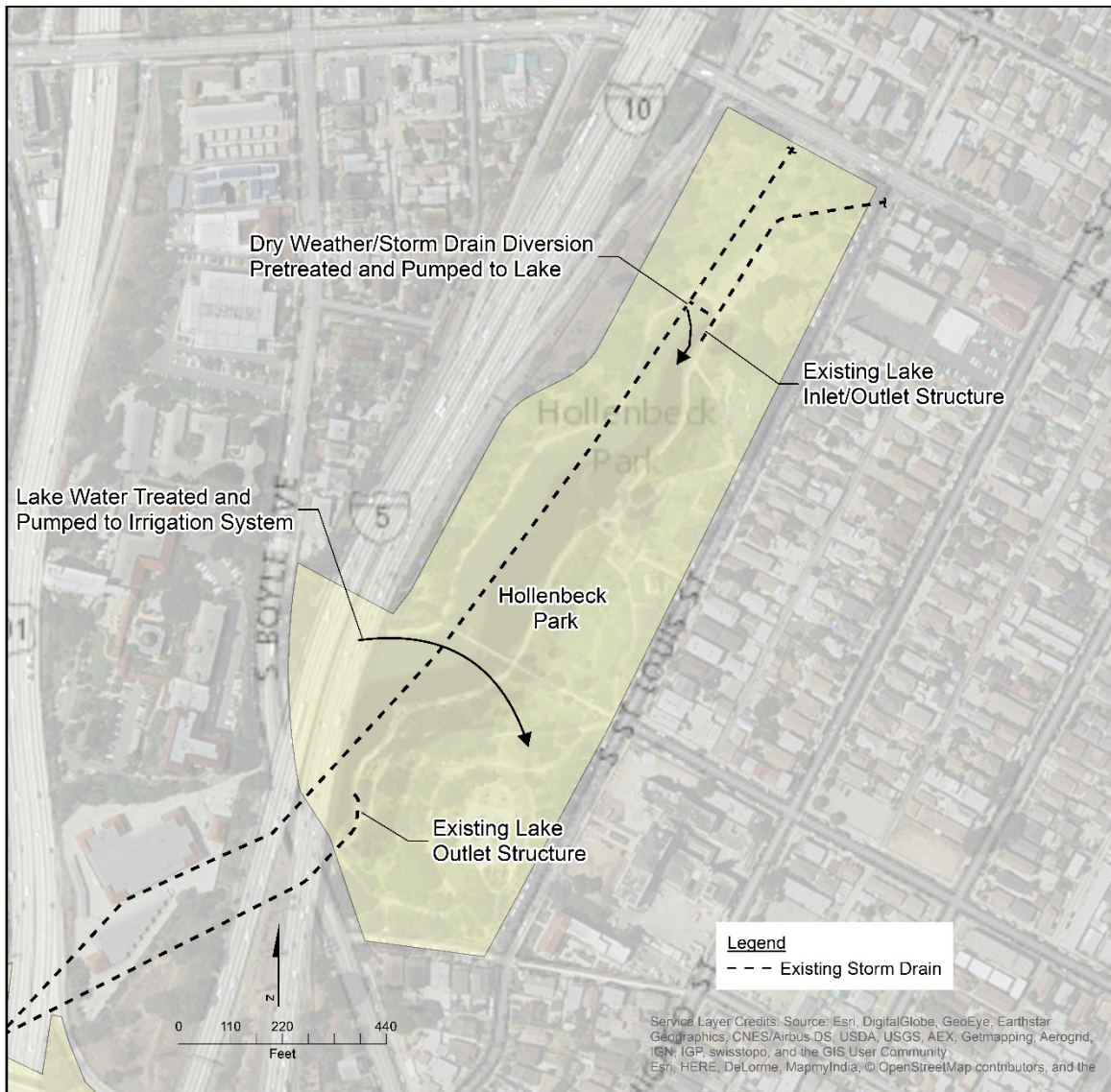
Figure 3-14. Conceptual Conveyance Alignment, Water Supply Alternative: HPL Overflows Hollenbeck Park Lake Rehabilitation and Stormwater Management
